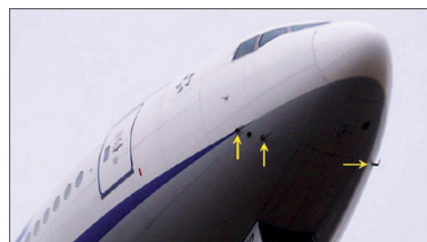
The aircraft’s speed sensors (known as “pitot tubes”) are located under the nose of the plane. If they ice over, as happened during the doomed Air France 447 flight, the autopilot disengages and the crew needs to take control of the plane.
